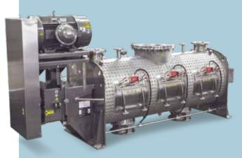
FKM Series batch mixers consist of a horizontal mixing cylinder with mixing elements mounted to the main shaft, a charging port located on top of the mixer, contour access doors on the front of the mixer, and a contour discharge opening on the bottom of the mixer. Electrical controls are designed to meet your specific requirements.
